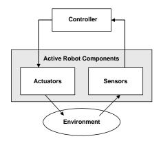
Figure 8. Mobile robot control loop architecture [40]
