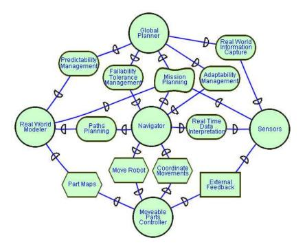
Figure 9. A structure-in-5 mobile robot architecture
