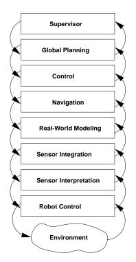
Figure 7. Mobile robot layered architecture [51]
